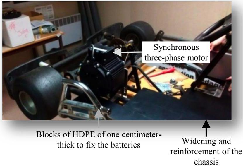
**Fig. 2.** Lightering, widening and reinforcement of the chassis
