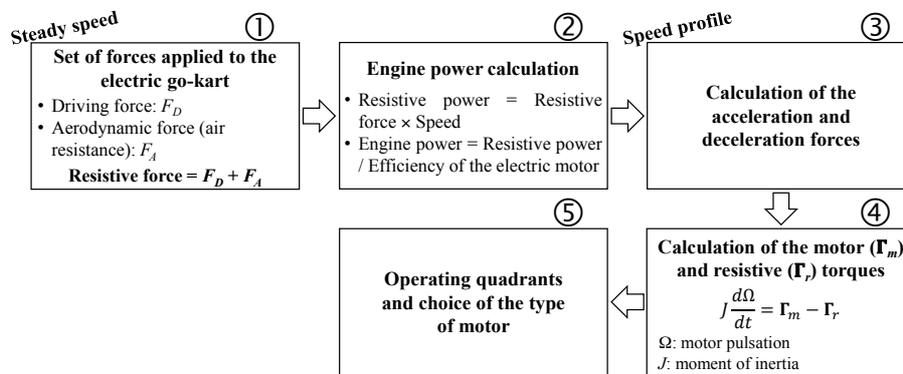
Fig. 1. Five main steps necessary to size the electric motor
