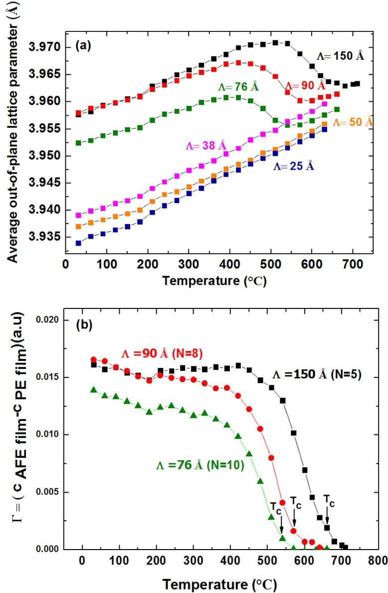
Figure 8: (a) Average out-of-plane lattice parameter versus temperature for all  $(\text{BiFeO}_3)_{0.5\Lambda}/(\text{LaFeO}_3)_{0.5\Lambda}$  superlattices and (b) corrected out-of-plane lattice parameter versus temperature for only  $\Lambda \geq 76$  Å SLs showing a structural phase transition.
