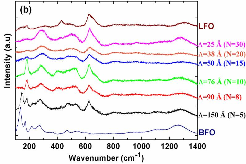
Figure 6: Room temperature Raman spectra of  $(\text{BiFeO}_3)_{0.5\Lambda}/(\text{LaFeO}_3)_{0.5\Lambda}$  superlattices in (a) parallel  $Z(\text{XX})\bar{Z}$  and (b) crossed geometry  $Z(\text{XY})\bar{Z}$ .
