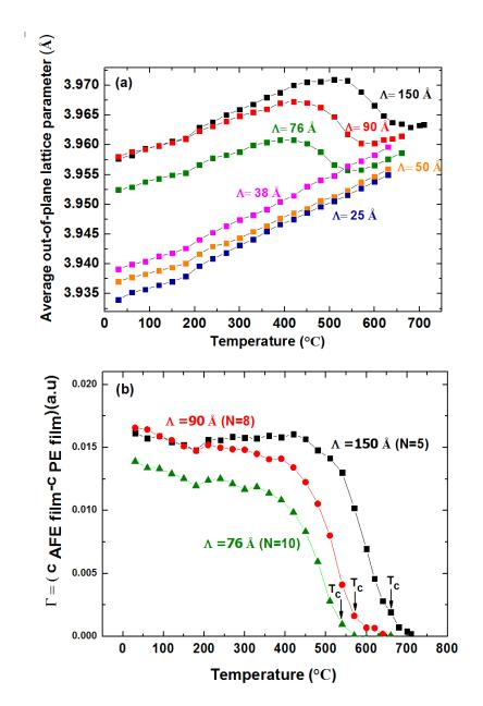
Figure 8: (a) Average out-of-plane lattice parameter versus temperature for all (BiFeO<sub>3</sub>)<sub>0.5 $\Lambda$ </sub> /(LaFeO<sub>3</sub>)<sub>0.5 $\Lambda$ </sub> superlattices and (b) corrected out-of-plane lattice parameter versus temperature for only  $\Lambda \ge 76$  Å SLs showing a structural phase transition.
