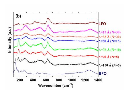
Figure 6: Room temperature Raman spectra of (BiFeO<sub>3</sub>)<sub>0.5 $\Lambda$ </sub> /(LaFeO<sub>3</sub>)<sub>0.5 $\Lambda$ </sub> superlattices in (a) parallel  $Z(XX)\bar{Z}$  and (b) crossed geometry  $Z(XY)\bar{Z}$ .
