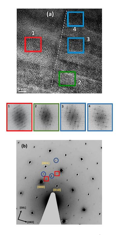
Figure 4: (a) High resolution TEM image for SL with  $\Lambda$ = 150 Å (N=5). The red square indicates the 45° dense lamellar only present in the BFO layers (periodicity of 1.15 nm), the green square shows any regions which reveal no domain structure in the BFO layers suggesting a pseudo-cubic unit cell. The blue squares highlight the horizontal and vertical
