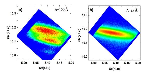
Figure 3: (204) Reciprocal space mapping of the SLs for (a)  $\Lambda = 150$  Å and (b)  $\Lambda = 25$  Å.
