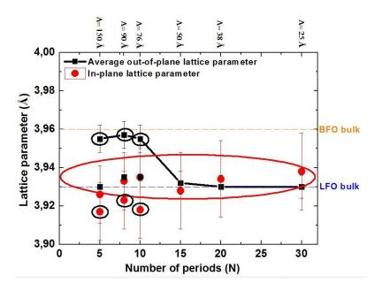
Figure 2: Lattice parameters calculated for all SLs. From  $\theta$ -2 $\theta$  XRD patterns: average out-of-plane lattice parameter (black squares symbol with line) calculated from the position of the most intense satellite peak. The out-of-plane lattice parameter (black squares only) calculated from the position of the second diffraction peak near the main reflection (see red
