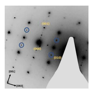
Figure 5: [100] ZAPD obtained for  $\Lambda$ =25Å (N=30) SL showing only Pnma-like reflections (½ {001} indicated by blue circles).
