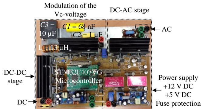
Figure 6. Prototype of the bidirectional DC-AC converter.
