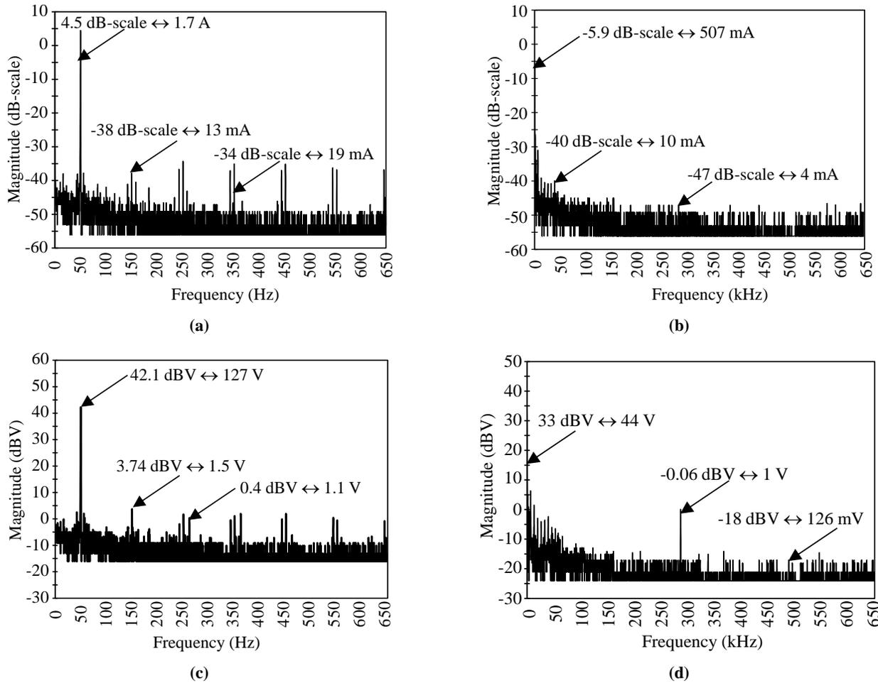
**Figure 8. Harmonic spectra of the output signals in the inverter mode (experimental results): (a) Output current at low frequency; (b) Output current at high frequency; (c) Output voltage at low frequency; (d) Output voltage at high frequency.**
