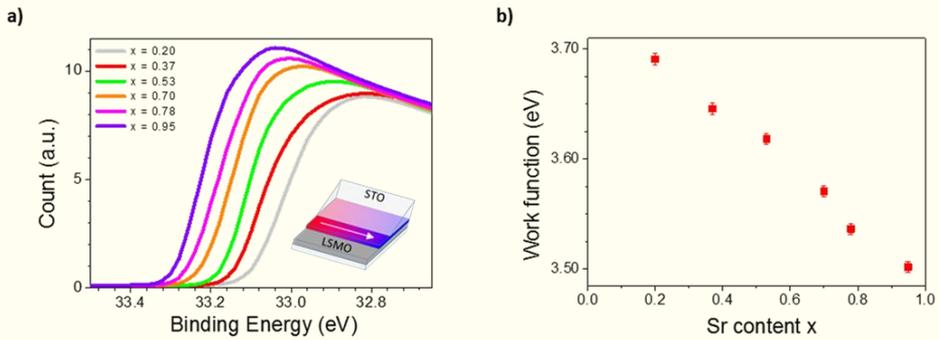
Figure 10: a) HeII UPS threshold for various  $x$  of air-exposed  $\text{LSMO}_x$   $U_{\text{bias}} = 4\text{V}$ . b) Corresponding extracted  $W_F$  versus Sr content  $x$
