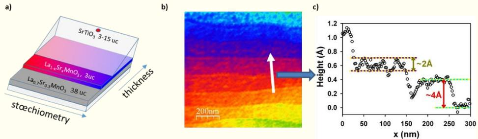
Figure 9: Schematic of the STO (sub.)/ LSMO / LSMO<sub>x</sub> / STO heterostructure. b) UHV-AFM image. c) Profile from the white arrow in b).
