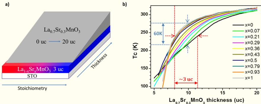
Figure 8: a) Schematic representation of the ICPLD LSMO<sub>x</sub> / wedge LSMO sample. b) Curie temperature curves versus  $t_{\text{LSMO}}$  for various Sr content  $x$  in LSMO<sub>x</sub> layer
