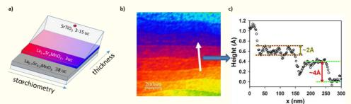
Figure 9: Schematic of the STO (sub.)/ LSMO / LSMOx / STO heterostructure. b) UHV-AFM image. c) Profile from the white arrow in b).
