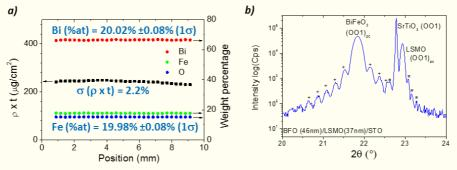
Figure 2: a) Evolutions of density × thickness product ( $\rho$ ·t) and weight percentages of Bi, Fe and O as a function of the position and b) X-Ray diffraction pattern of BFO/LSMO/STO heterostructure
