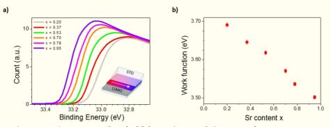
Figure 10: a) HeII UPS threshold for various x of air-exposed LSMO<sub>X</sub>  $U_{\text{bias}} = 4V$ . b) Corresponding extracted  $W_F$  versus Sr content x
