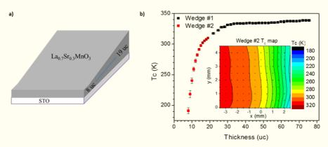
Figure 7: a) Schematic of LSMO wedge#2. b)  $T_C$  versus thickness and (inset)  $T_C$  map for wedge #2
