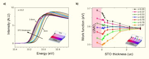
Figure 11: a) HeII UPS threshold for various  $t_{STO}$  at x=0.2 U<sub>bias</sub> = 4V. b) Corresponding extracted W<sub>F</sub> versus  $t_{STO}$  for various Sr content x
