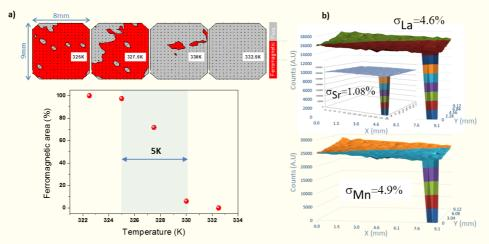
Figure 6: a) Magnetic state maps of LSMO 20 uc film at various temperature (top) and  $T_C$  distribution at the sample surface (bottom). b) WDS signal for La, Sr and Mn over 9x9 mm<sup>2</sup> of the same sample.
