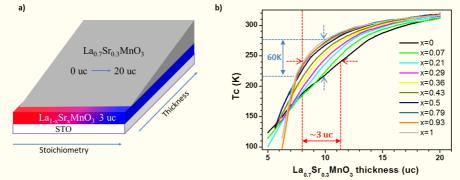
Figure 8: a) Schematic representation of the ICPLD LSMO<sub>x</sub> / wedge LSMO sample. b) Curie temperature curves versus  $t_{LSMO}$  for various Sr content x in LSMO<sub>x</sub> layer
