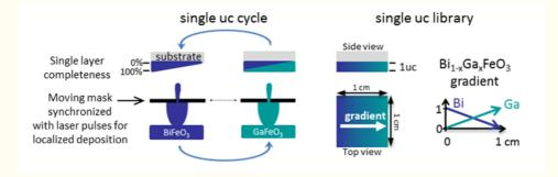
Figure 1: Schematic of the combinatorial single layer synthesis and of the resulting composition spread library (e.g.  $Bi_{1-x}Ga_xFeO_3$  composition library)
