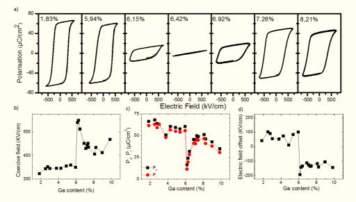
Figure 4: a) Ferroelectric cycles for various Ga contents measured at 77K. The corresponding coercive fields, remanent and saturation polarizations and electric field offsets are plotted in b), c) and d) respectively
