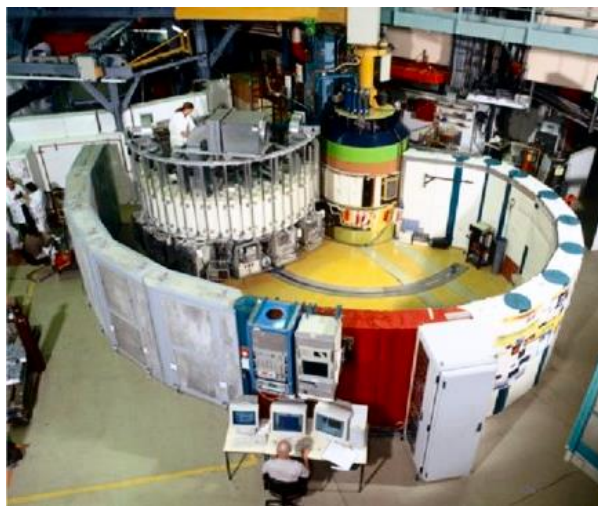
Fig. S1 D20 –High Intensity two-axis diffractometer located at the Institut Laue–Langevin (ILL-Grenoble) reactor hall, thermal beam H11.
