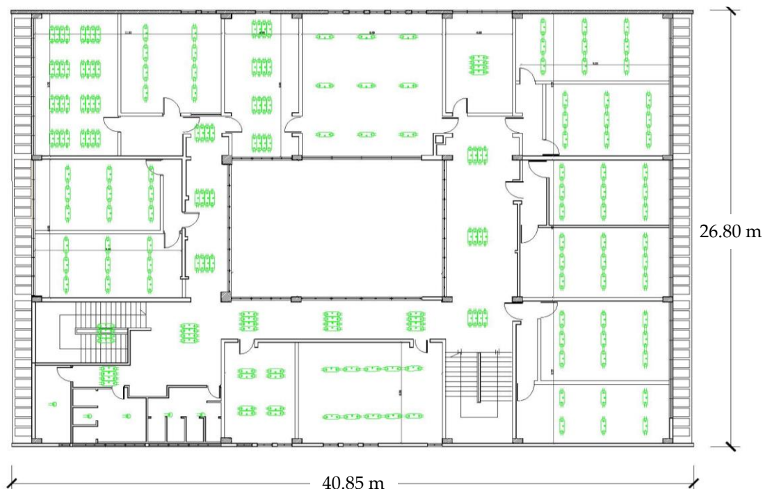
Figure 5. Existing light fixtures (in green) in the building studied.
