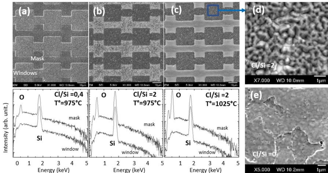
**Figure 2.** SEM images recorded on SiO<sub>2</sub> masked 3C-SiC(100) surface after Si growth under different conditions. EDS spectra recorded both on mask and window regions. (d)-(e) SEM on chlorinated - non-chlorinated growth respectively.
