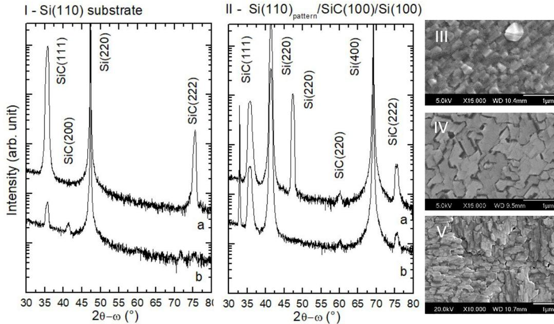
**Figure 3.** XRD (I) SiC on Si substrate: (a) intro 870°C, (b) intro 930°C; (II) SiC on heterostructure: (a) non-annealed, (b) annealed; SEM on  $C_3H_8$  intro 930°C surface (III),  $C_3H_8$  intro 870°C (IV), heterostructure (V).
