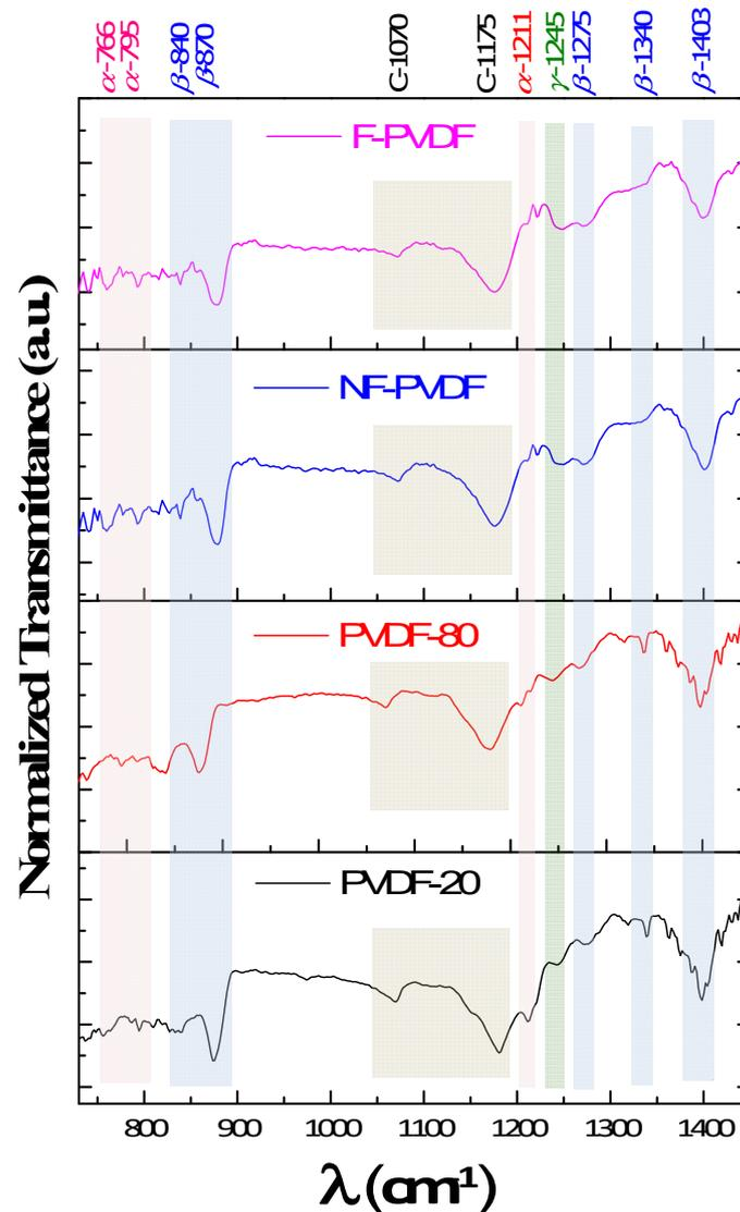
**Figure 2.** Infrared absorption bands typical of the  $\beta$  and  $\alpha$  phases were identified, and they are presented separately for neat PVDF films (PVDF-20 and PVDF-80) and hybrid ones with non-functionalized nanoparticles (NF-PVDF) and functionalized nanoparticles (F-PVDF).
