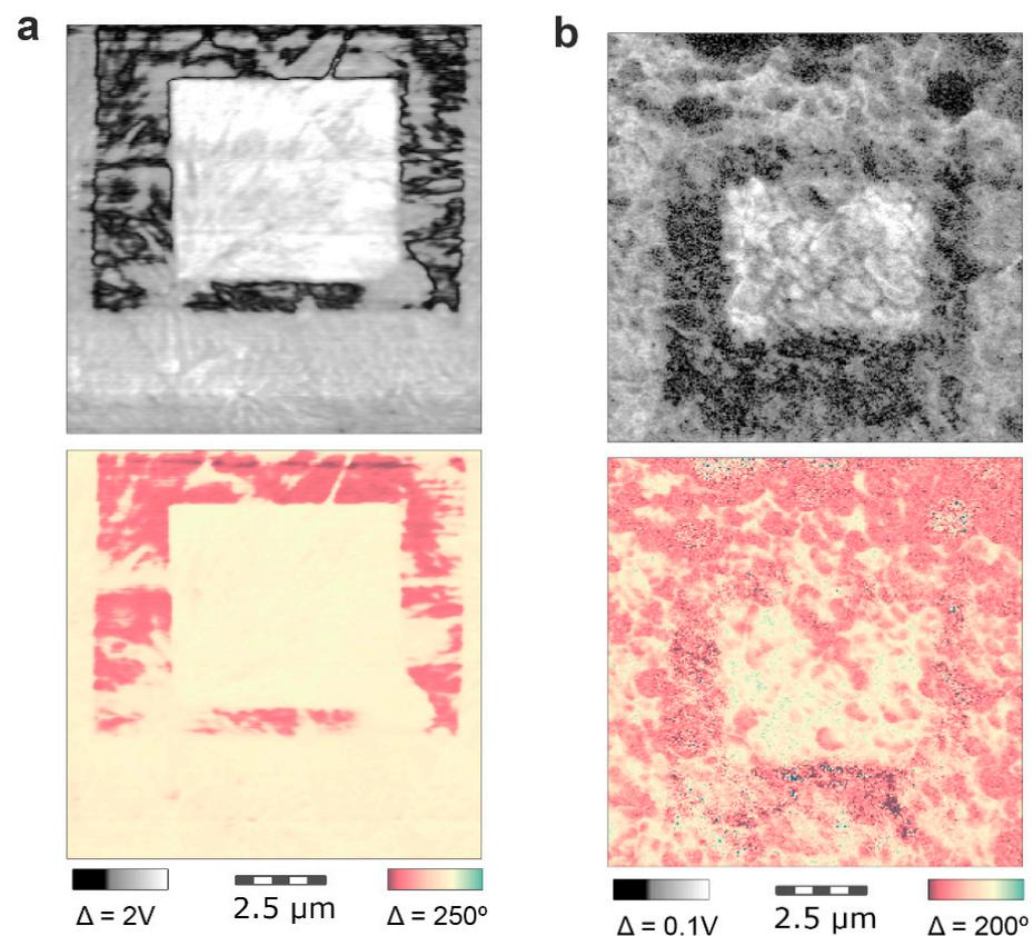
**Figure 6.** (a) PFM amplitude (top) and phase (bottom) of the PVDF-20 film 24 h after the polarization process and image scanning; (b) PFM amplitude (top) and phase (bottom) of the F-PVDF film 24 h after the polarization process and image scanning.
