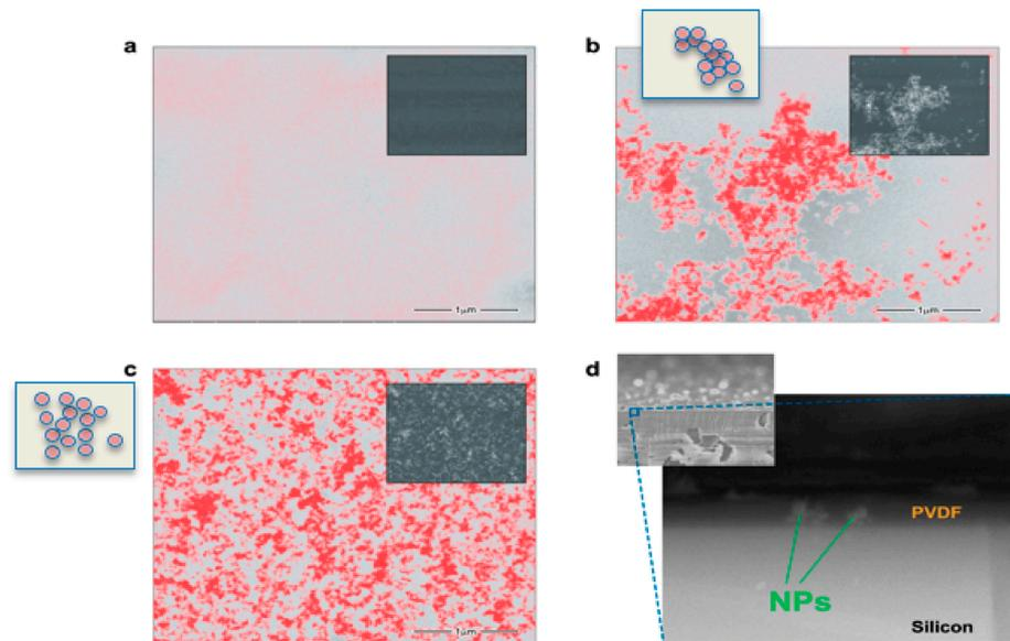
**Figure 4.** SEM images of (a) a neat PVDF film; (b) non-functionalized NPs embedded in the PVDF film (NF-PVDF); (c) functionalized NPs embedded in the PVDF film (F-PVDF); (d) cross-sectional image of the NF-PVDF sample. The scale bar in (a–c) is 1  $\mu\text{m}$ .
